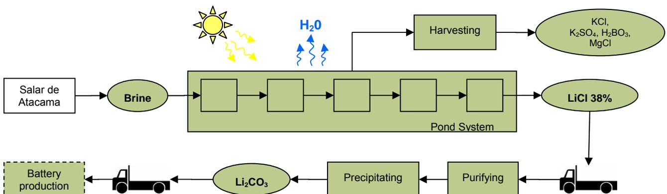
**Figure 1:** Flowchart of the processes considered in the LCI of lithium extraction (Salar de Atacama, Chile) and further processing to  $\text{Li}_2\text{CO}_3$
