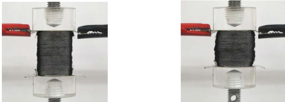
**Figure 19.** DE stack actuator equipped with fixed end parts: deactivated (left) – activated (right)
