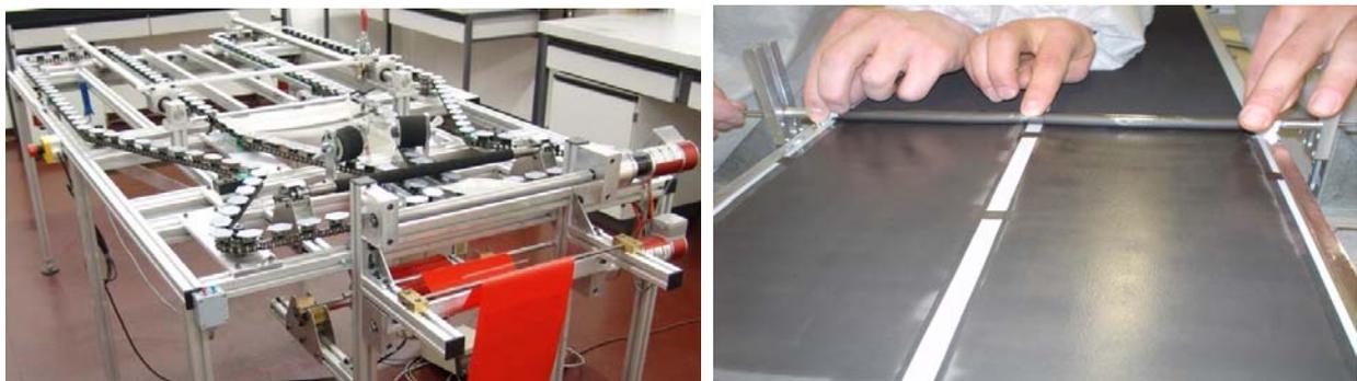
**Figure 13.** Film pre-stretching machine (left) – rolling process of the pre-stretched film (right)
