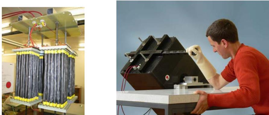
**Figure 9.** The four actuator banks (left) placed inside of the arm wrestling robot (right)
