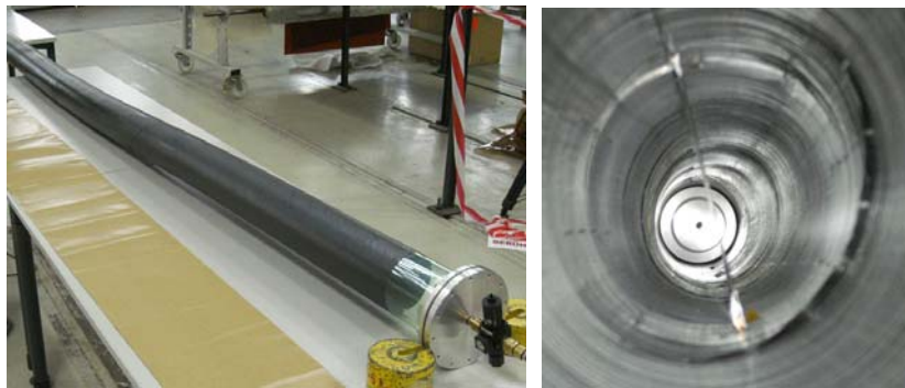
Figure 13. Breadboard of the deployable/inflatable boom with DEAs 13. (Courtesy of High Performance Space Structure Systems GmbH)
