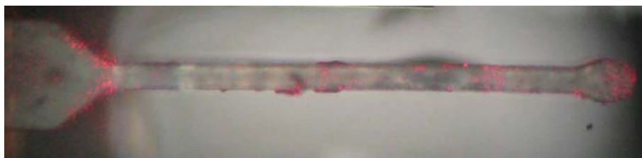
Figure 8. Top view of optical waveguide cantilever, the length of the beam is 450 \mu m from the support to the tip.
