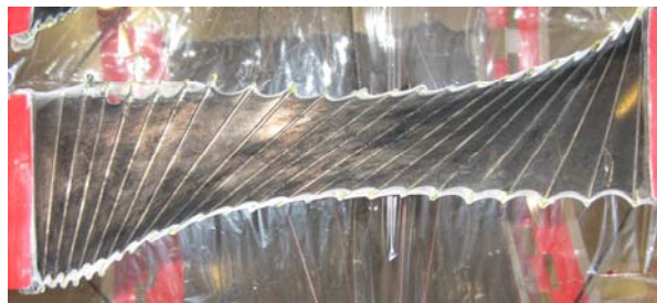
Fig. 11: Instability of the reinforcing rods.
