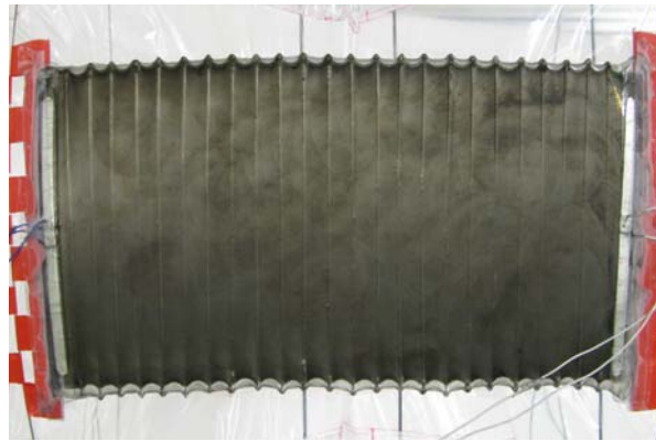
Fig. 5: Actuator design with internal reinforcement
