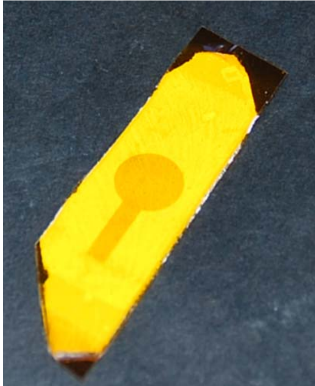
Figure #1. Photograph of a 1 mm thick slice of PVDF foam sandwiched between two layers of polyimide tape with patterned platinum electrodes. Samples like these were used in the charge and piezoelectric measurements.
