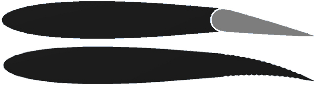
Figure 1: Aerofoil with conventional hinged (top) and variable camber corrugated control surface (bottom)
