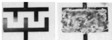
Fig.2. Interdigitated electrodes. (a) without PANI, (b)with PANI
