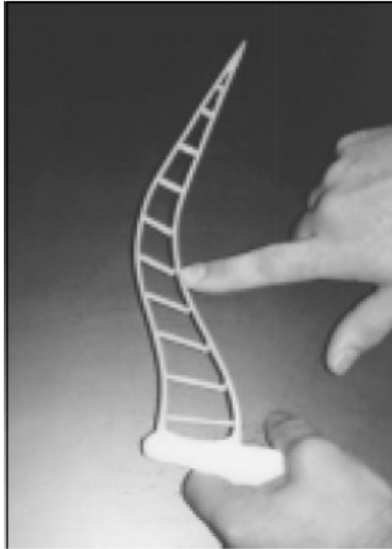
Figure 6. Demonstration of the Fin Ray Effect®.
