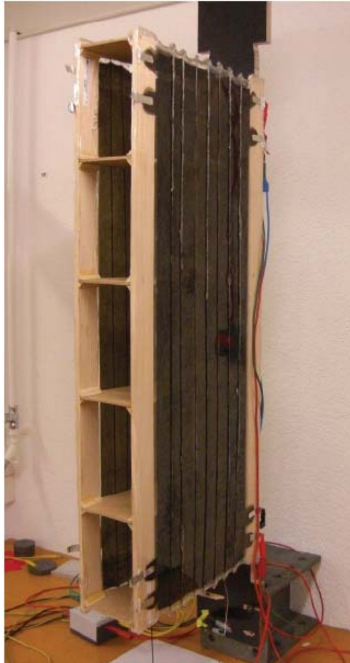
Figure 11. Full size functional model of the active hinge for the activation of the tail fin.
