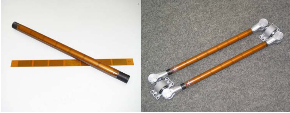
Figure 7. Rods for Triglide . Left side: single patch-actuator and rod, right side: complete link built of two rods
