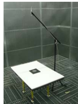
Figure 3. Measuring SPL in an anechoic chamber.
