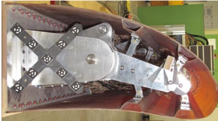
Figure 13: SADE Kinematic Station in WT Demonstrator (deployed position)
