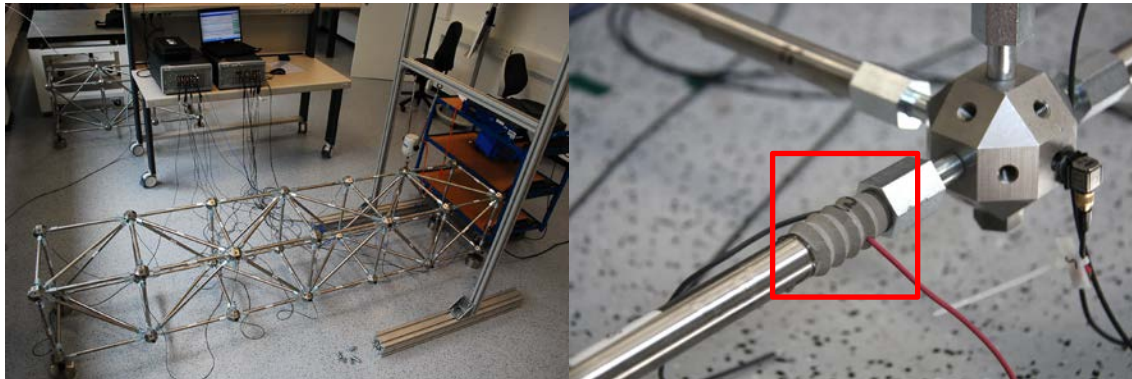
Figure 4: Truss structure (left) and installed active strut between nodes 18 and 19 (right)
