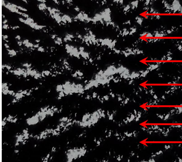
Figure 9. Backlit 10mm thick sample. Particles are dark with a light background. Distinct banding spaced approximately 1mm apart is highlighted with red arrows. Sample subjected to both the magnetic field pictured in Figure 5 and 50 \mu m vibration at 300Hz.
