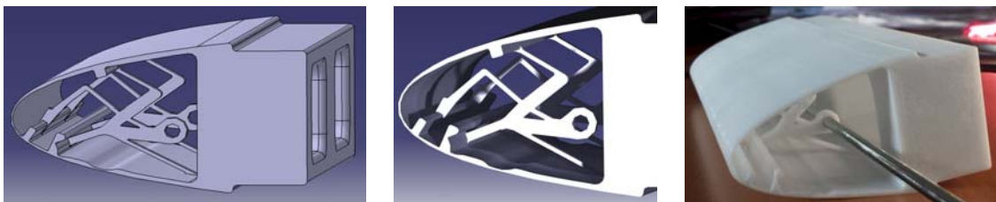
Figure 11. Production sequence of a morphing LE based on FDM technology.
