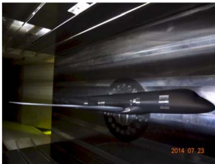
Figure 5. The RA model inside the CSIR transonic wind tunnel.
