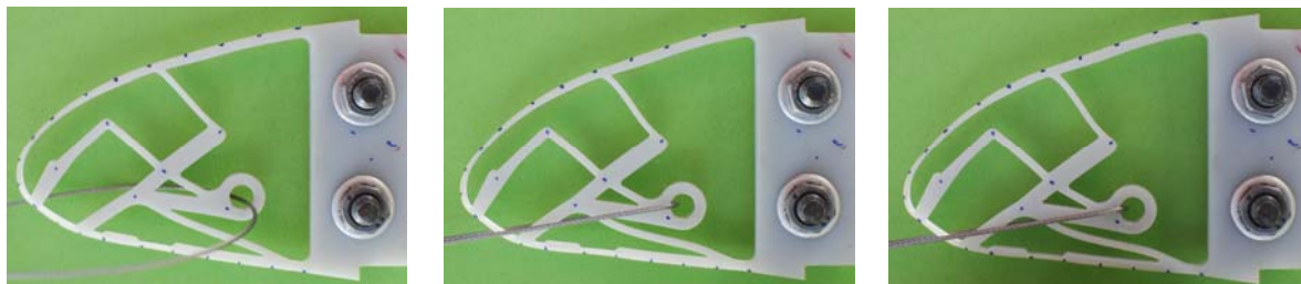
Figure 12. Preliminary static test on a morphing rib manufactured by Polyjet technology: unloaded structure (left), intermediate load (middle) and maximum load (right).
