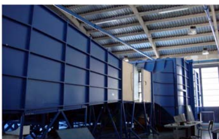
Figure 6. The wind tunnel used for morphing devices validation at POLIMI.
