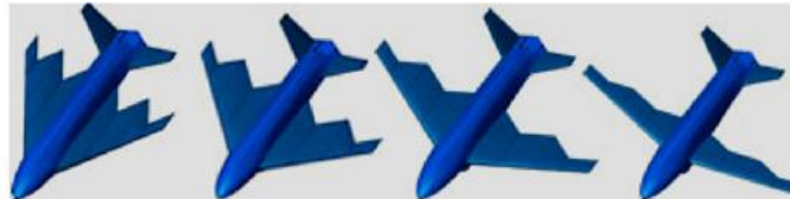
Figure 1. Biologically inspired morphing aircraft: sliding skin (Raytheon, sweep angle changes) [3]
