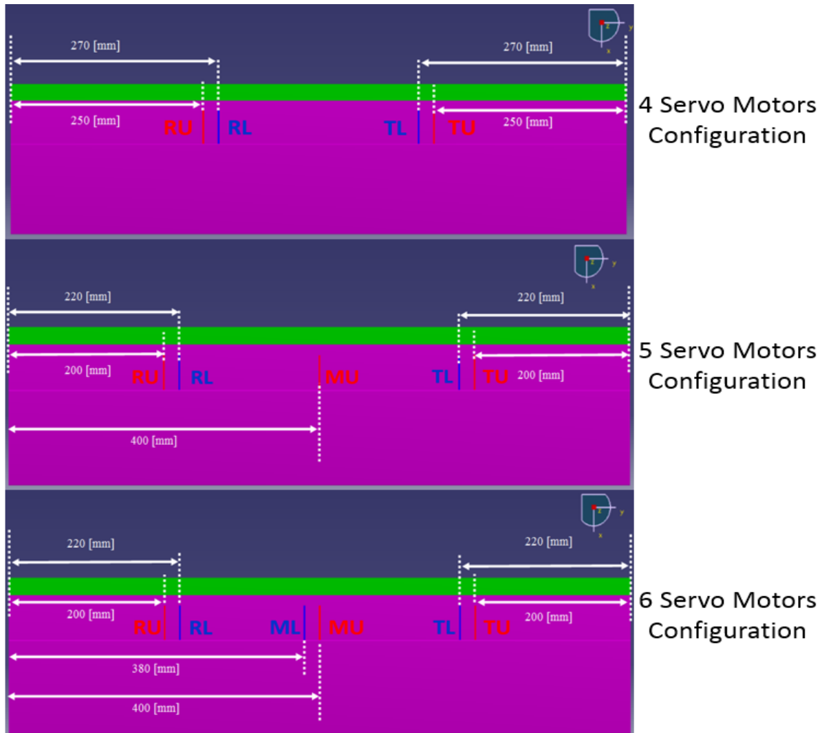
Figure 9. Locations of the Servo Motors. The Servo Motors that actuate the Upper Surface are shown in Red and the Lower Surface are shown in Blue
